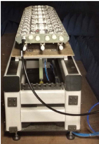
Fig. 21. Proposed antenna is tested on PIM 3 .
